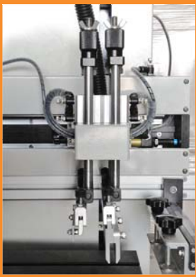
Squeegee & Floodbar Assembly with micro adjustability
