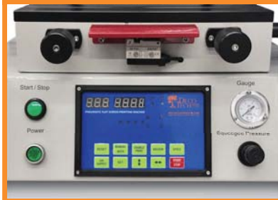
Close Up View of the Control Panel with Membrane Switches & LCD Display
