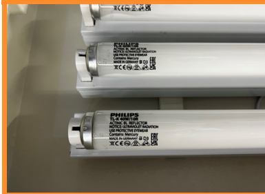
Close-up of 40W UV Fluorescent Tubes
